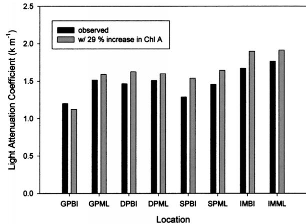
Fig. 5. Observed mean light attenuation coefficients ( $\text{k m}^{-1}$ ) and predicted light attenuation coefficients with a 29% increase in chlorophyll *a* concentrations for all sites (see text). GPBI = Gasparilla Pass Barrier Island, GPML = Gasparilla Pass Mainland, DPBI = Don Pedro Barrier Island, DPML = Don Pedro Mainland, SPBI = Stump Pass Barrier Island, SPML = Stump Pass Mainland, IMBI = Indian Mound Barrier Island, and IMML = Indian Mound Mainland.
