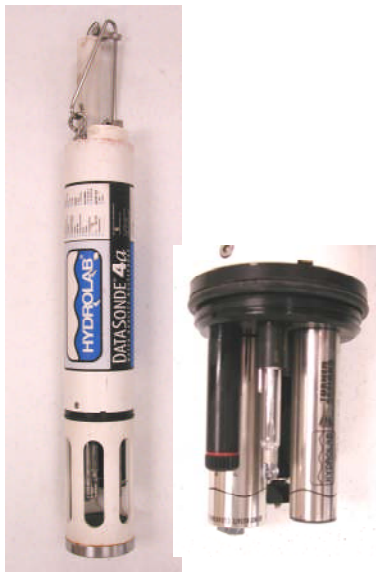
Figure 39. Hydrolab sonde (L) and a close up of the sensors (R).
