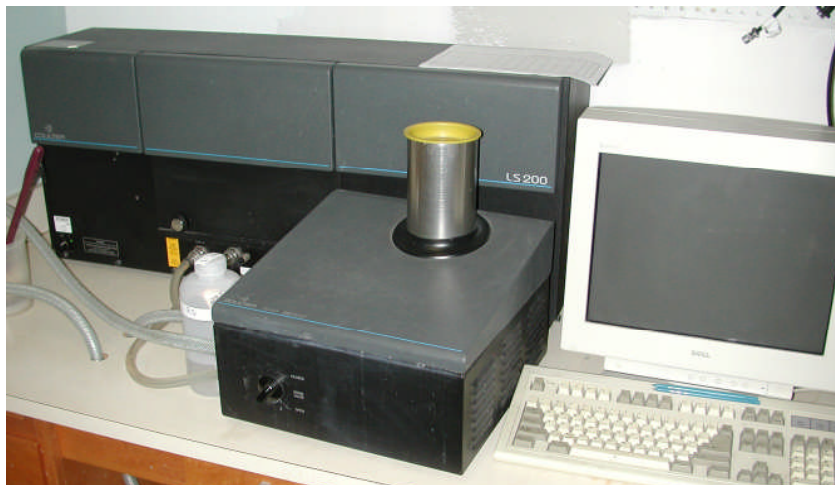
Figure 44. Coulter LS 200 particle size analyzer.
