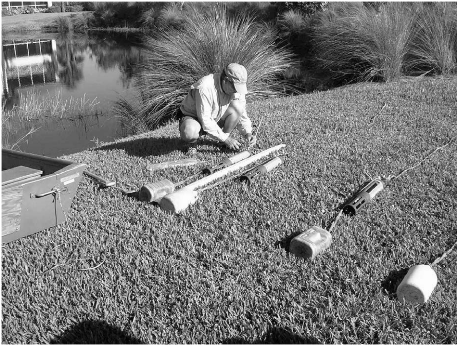
FIG. 5. Deep and Shallow Stormwater Pond Aeration Study Aeration Study at The Brooks Showing the submersible datasondes used in the study.
