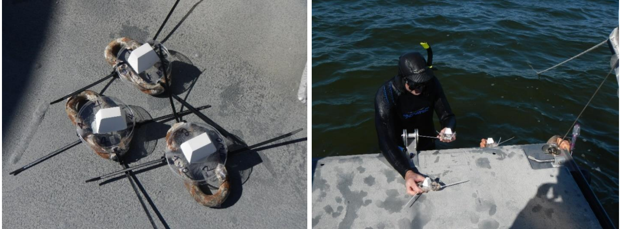
Figure 6. Clod cards used to estimate relative flow rate between sites. Images show three cards ready to deploy and manual deployment by divers to base of float and block.
