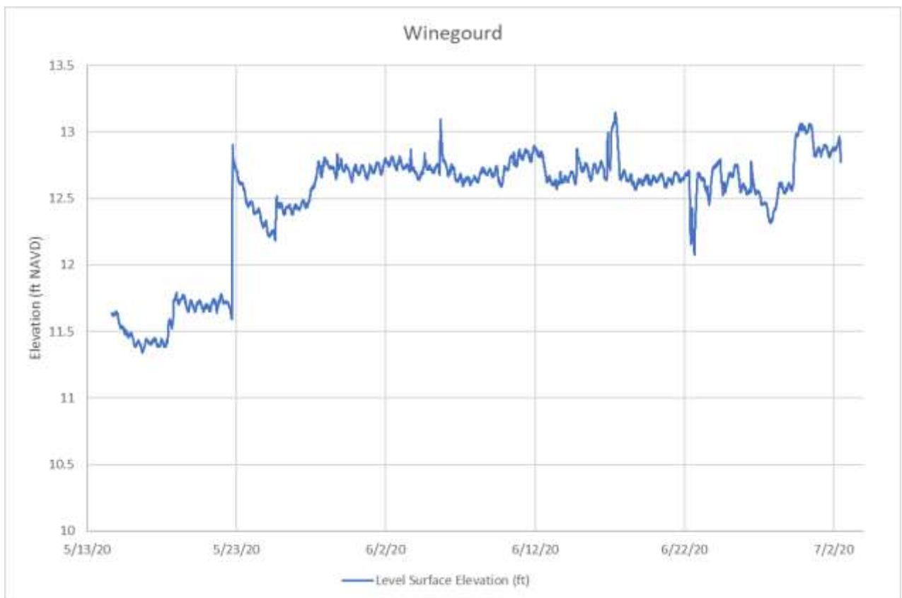
Figure 24- Surface water elevation for flow monitoring station Winegourd Creek measured in ft-NAVD
